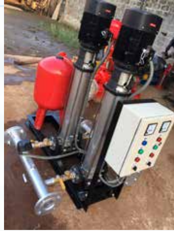
Horizontal multi-stage pump with pressure tank used for booster operations
