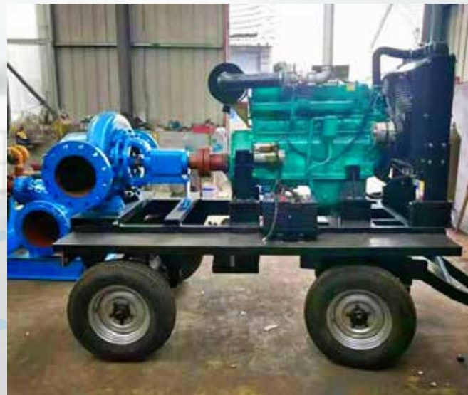
Mobile booster pump for irrigation and other purposes
